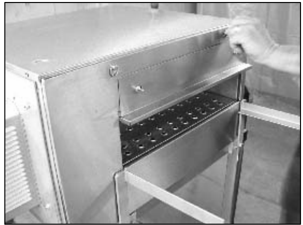
20. Install the infeed end cover by lining up the slots at the bottom of the end cover with the brackets on the oven and push in on the latches and turn clock wise.
